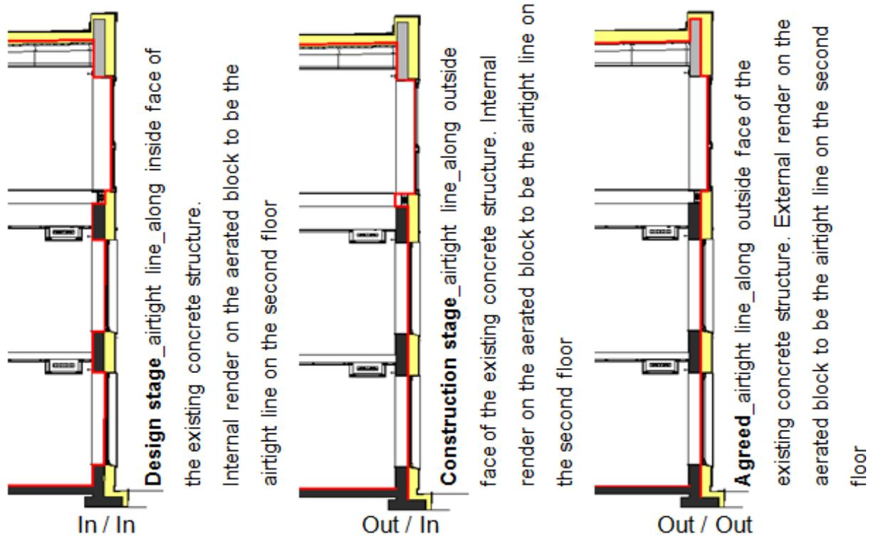
Figure 5: Typical section showing airtight line journey (not to scale)
