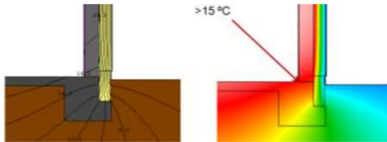
Figure 4: Refurbished existing foundation thermal bridge analysis using Therm software (not to scale)
