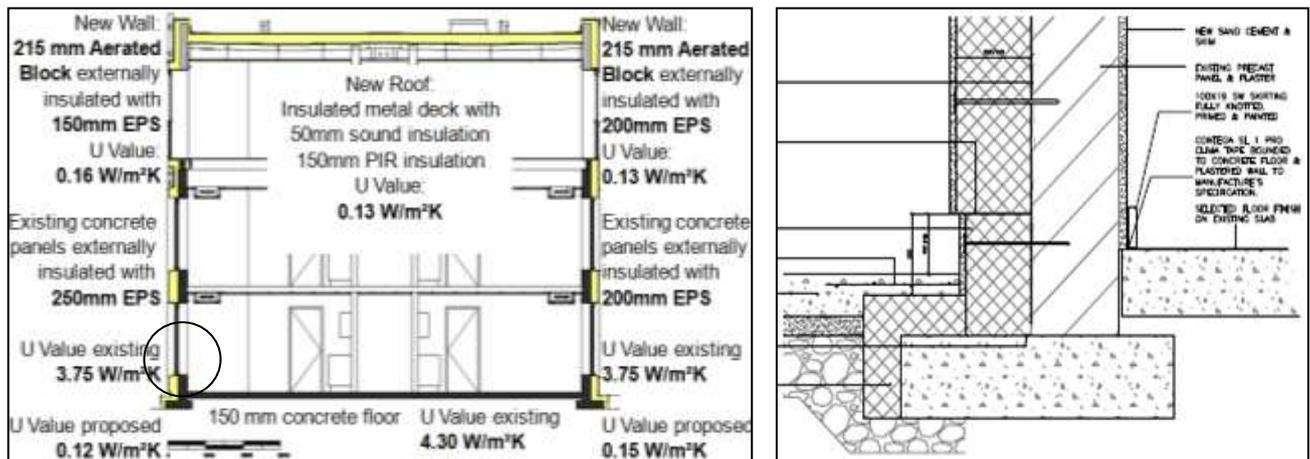
**Figure 3: Left: Typical section showing two lower existing floors with new second floor above and the proposed external insulation on existing walls and new walls, indicating U-values of existing and proposed EnerPHit development (MosArt 2015) (not to scale). Right: Existing foundation detail showing the proposed external insulation on existing external walls down to the foundation and wrapping down to the edge of the foundation foot (Source: DLR Co. Co.) (not to scale)**
